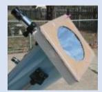
While there are many commercial solar filters for telescopes, it is also possible to make your own filter. In order to safely observe the sun with a telescope, you must have a
