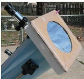
**BUILD A SAFE SOLAR FILTER** for your telescope, binoculars or camera. You can make your own Safe Solar Filter using a sheet of Mylar Baader coated material from AstroPhysics. This specially designed material gives safe images with excellent resolution. The Astronomy Club of Tulsa has ordered some of the material in bulk.
