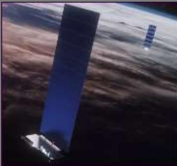
**S&T** SpaceX has begun launching a mega-constellation of 1,584 Starlink satellites into 24 orbit plain – 66 per plain. They have also applied to the FCC to move the same number of satellites into 72 orbit plains. The satellites are designed to provide Broad Ban Internet service to the many rural or 3<sup>rd</sup> world regions that have no service.
