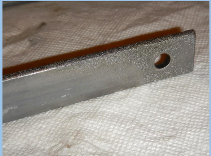
Bracket, After 12-hour Soak in Evapo-Rust
