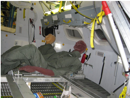
# 2 Enigineering Mock-up with mannequins placed in the pilot positions. Note the three panel display suspended over the astronauts
