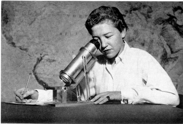
The convenience of table-top observing is illustrated by this picture of Miss Marjorie Holt using an experimental MOONWATCH telescope constructed in the shops of the Smithsonian Institution. The mounting is made entirely of aluminum. The telescope's bed-plate has a rigid extension inclined at 45 degrees to carry the front-surface mirror.
