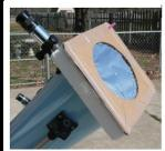
BUILD A SAFE SOLAR FILTER for your telescope, binoculars or camera. You can make your own Safe Solar Filter using a sheet of Mylar Baader coated material from AstroPhysics. This specially designed material gives safe images with excellent resolution. The Astronomy Club of Tulsa has ordered some of the material in bulk.
